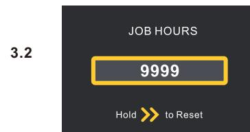
**“Indicates”:** Do I need to clear out this time? “>>” if you need to clear. When the operation is completed, the working time of the main interface and the working time of this interface will be reset and started to be instant again. After accumulation (9999), clean up and round.
