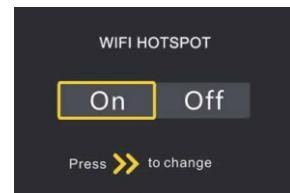
**3.4 Wifi hotspot**: factory setting is “OFF”, press > to enable wifi hotspot and switch ON/OFF. The device can transmit data and receive APP commands. The icon flickers when connected on the main interface. After successful connection, the icon displays normally.
