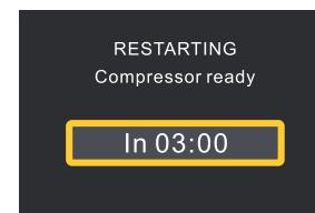
**“Compressor ready IN 03:00” indicates** : That the interface will be displayed when the compression is in a protected state. (including power-on and shutdown, the humidity rises immediately after the arrival of LO HI, and the shutdown resumes immediately after the emergence of LO HI). Displays the countdown in seconds. If the above situation does not occur within 3 minutes, it is not shown.
