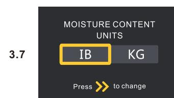
**3.7 MOISTURE CONTENT UNITS**: It is used to switch the unit of GPP value with moisture content. Press > to switch the lb or Kg, after switch symbol of corresponding parts is also changing.
